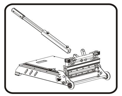
Installation of the Cutter(1) Install the handle assembly to the cutter base as shown.
