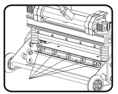
**Changing the Nylon Bar** Use provided Allen wrench to Loosen the five screws, then carefully move nylon bar out of the nylon bar holder.
